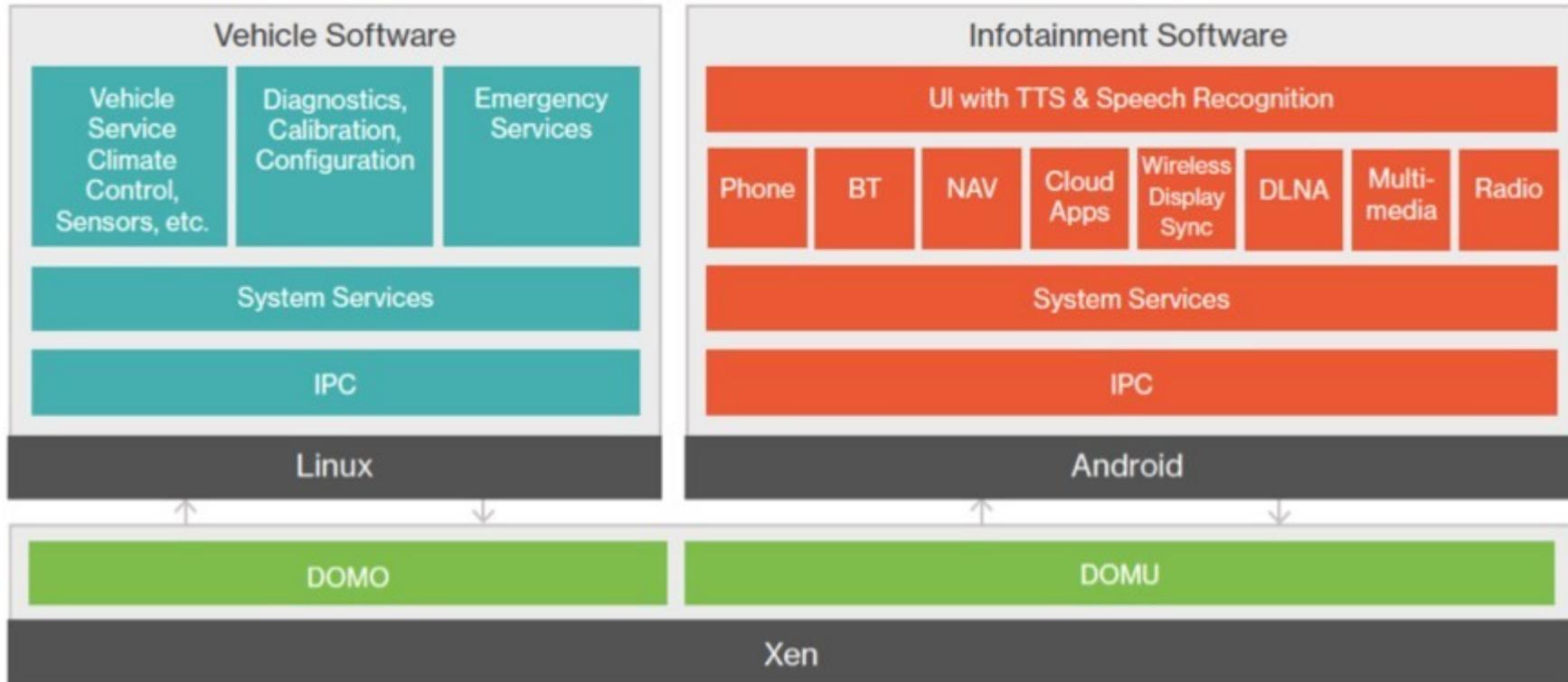
DOM0 and DOMU run on different cores of a processor.
