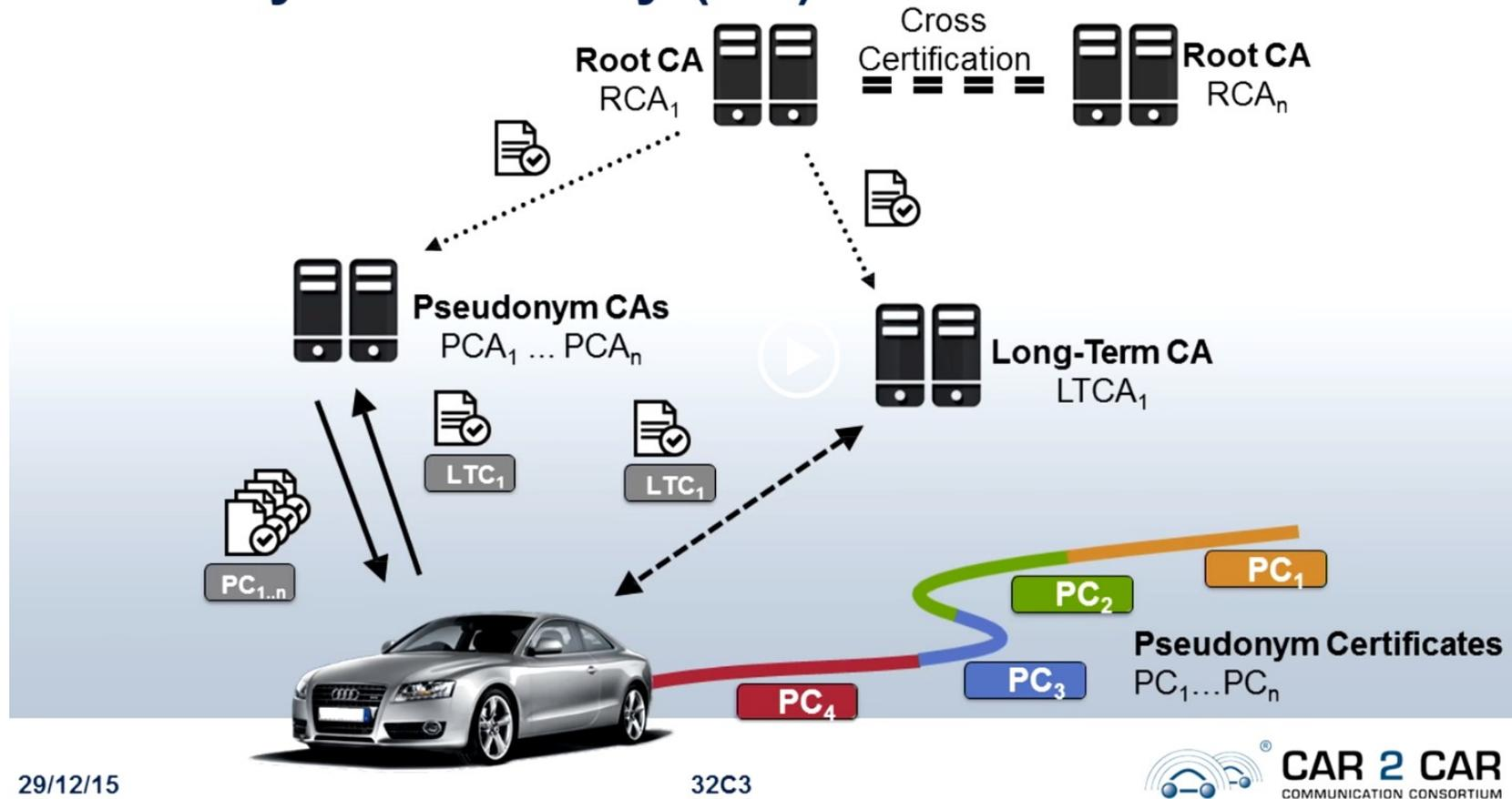
Courtesy B. Lehmman, 32C3, “Vehicle2Vehicle Communication based on IEEE802.11p”
