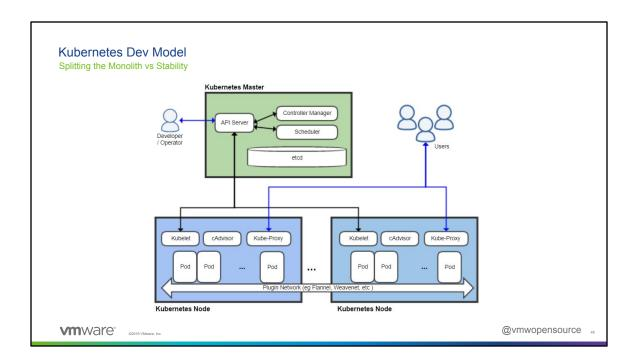
Old, dated architectural diagram of k8s control plane. Especially with most of the component code in one repo, it's easy to imagine validating this as an integrated cluster unit.
