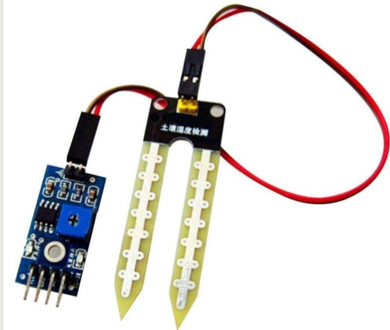
The soil motion sensor is used to determine the amount of moisture of the soil of the plant. This data is then taken into consideration when triggering the watering system.
