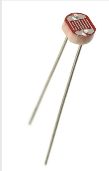
The photoresistor is used to measure how much light is being emitted on the plant. This data is used to determine whether the user would have to move the plant or not.
