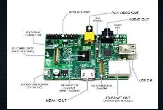
The Raspberry Pi is a small computer w/ 700 Mhz Single Core Atom and up to 512 Mb memory all for \$25 13
